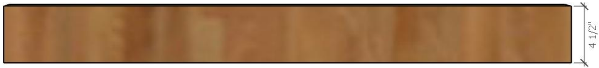
Figure 33: Piece of Wood Used for the Bottom-edge of the Collector Frame
