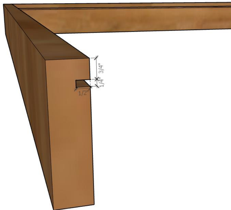
Figure 31: Location and Dimensions of the Notch Cut into the Collector
