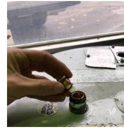
Figure 77: Removing the heat trap insert from the cold-water Inlet
