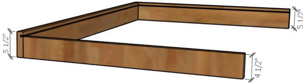
Figure 32: Three sides of the Collector Frame Assembled
