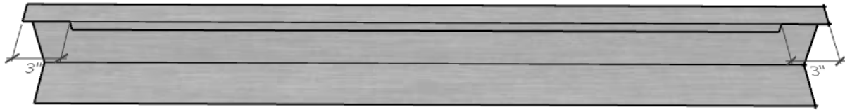
Figure 61: Notching the Ends of the Top Flashing
