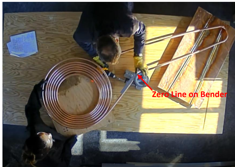
Figure 16: Pipe Bender on the Copper Pipe at the Start of the Second Bend
