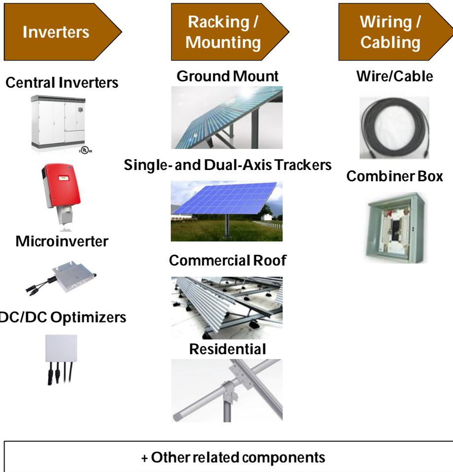
**Figure 11 – Balance of System Components**
