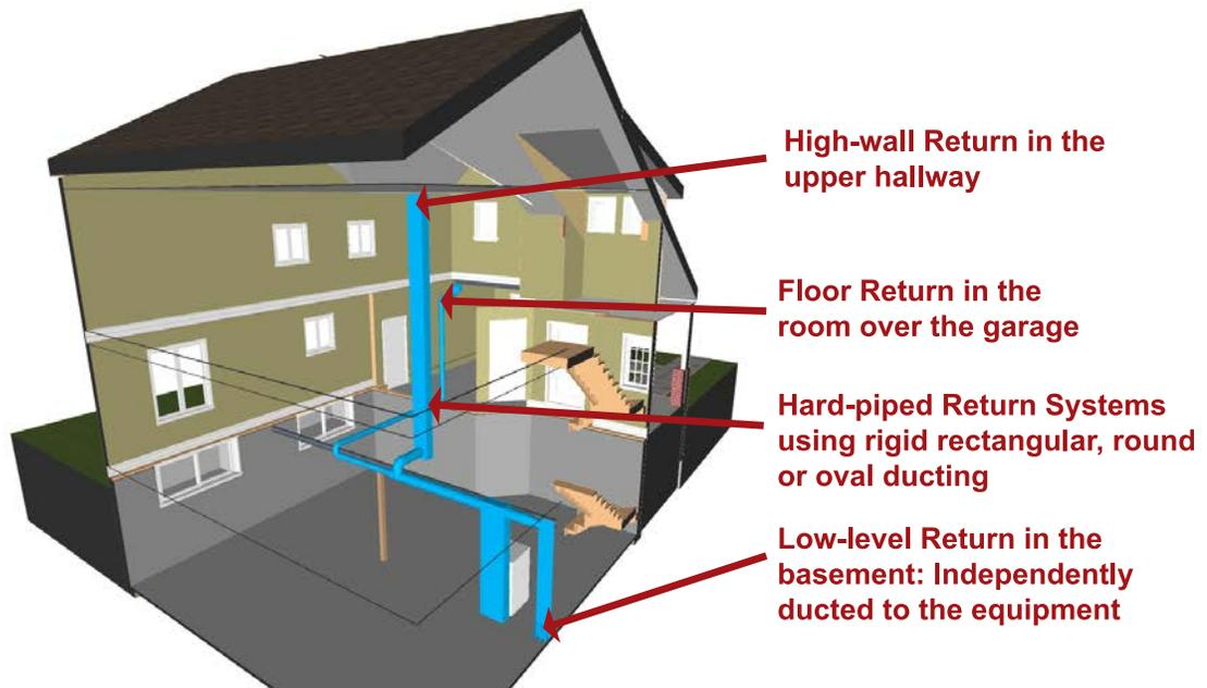
Figure 4-4: Example of a Simplified Return Duct System in a Two-Storey House
