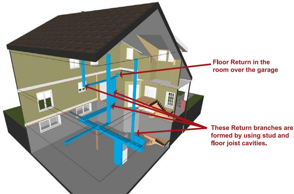
**Figure 4-1:** Example of a Standard Return Duct System in a Two-Storey House
