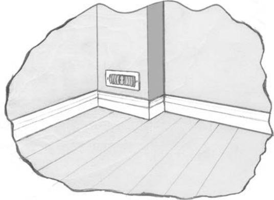
**Figure 5-4:** Perimeter Low Wall Supply Outlet
