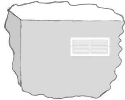
Figure 4-2: High Wall Return Inlet
