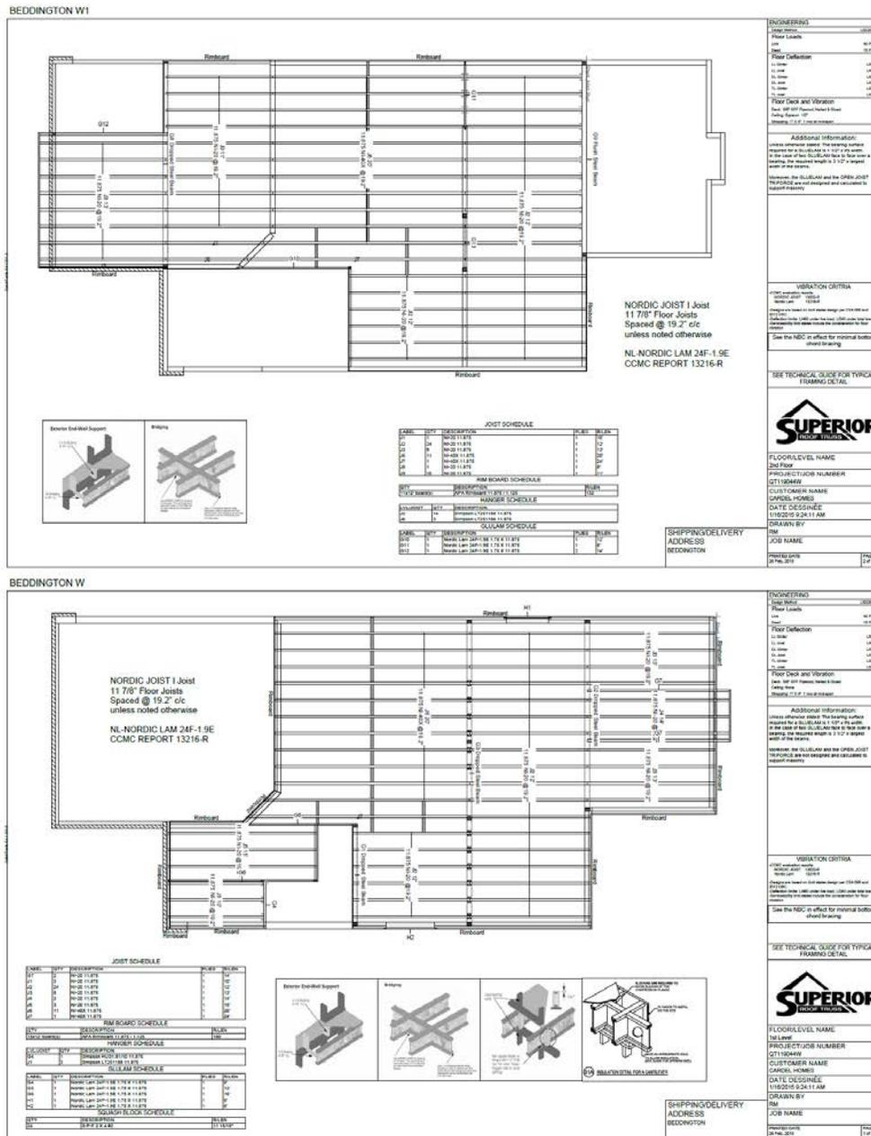
Figure B-20: Joist Plan Details to Assist with HVAC Duct Routing
