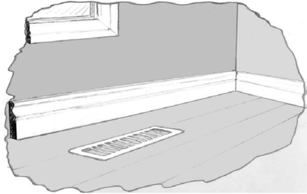
**Figure 5-1:** Perimeter Supply Outlet with Floor Diffuser
