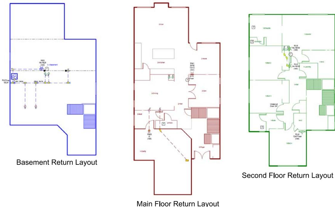
**Figure B-23:** Return duct layout for the Example Duct Design
