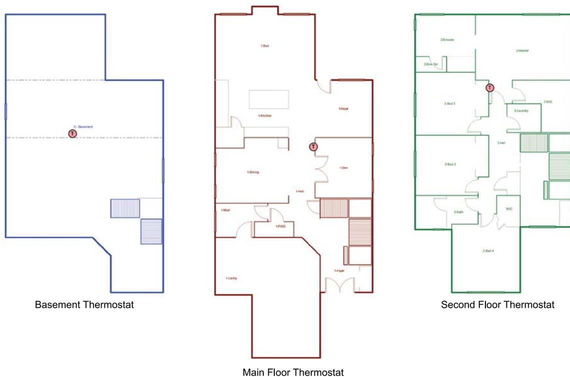
**Figure B-25:** Zone Thermostat Locations in the Example Three-Zone HVAC Design
