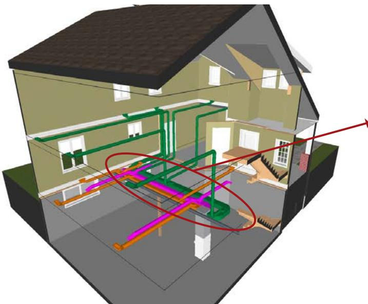
**Figure 5-11:** Supply Ducts for Basement, Main Floor and Second Floor Zones
