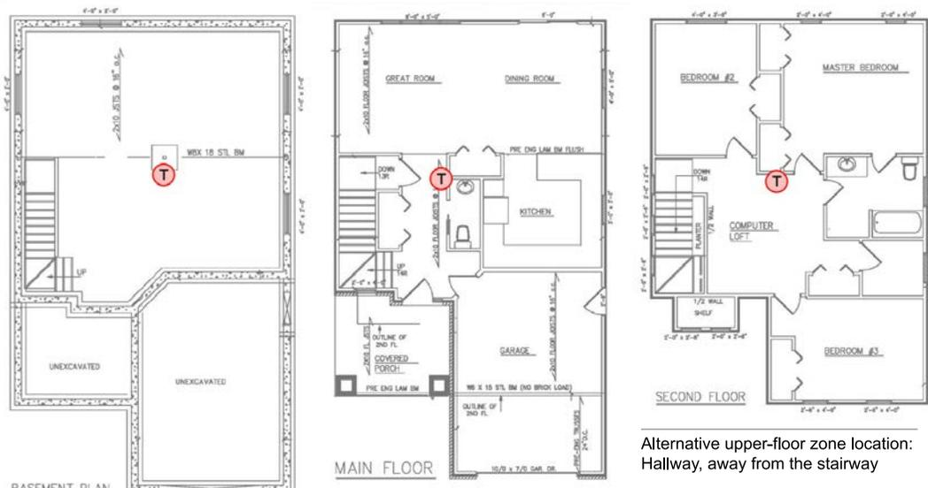
Figure 6-1: Hallway Thermostat Placement for a Three-Level Home, Zoned by Floor
