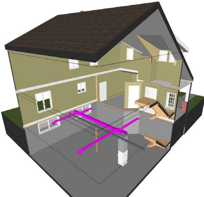
**Figure 5-9:** Supply Ducts for Basement Zone
