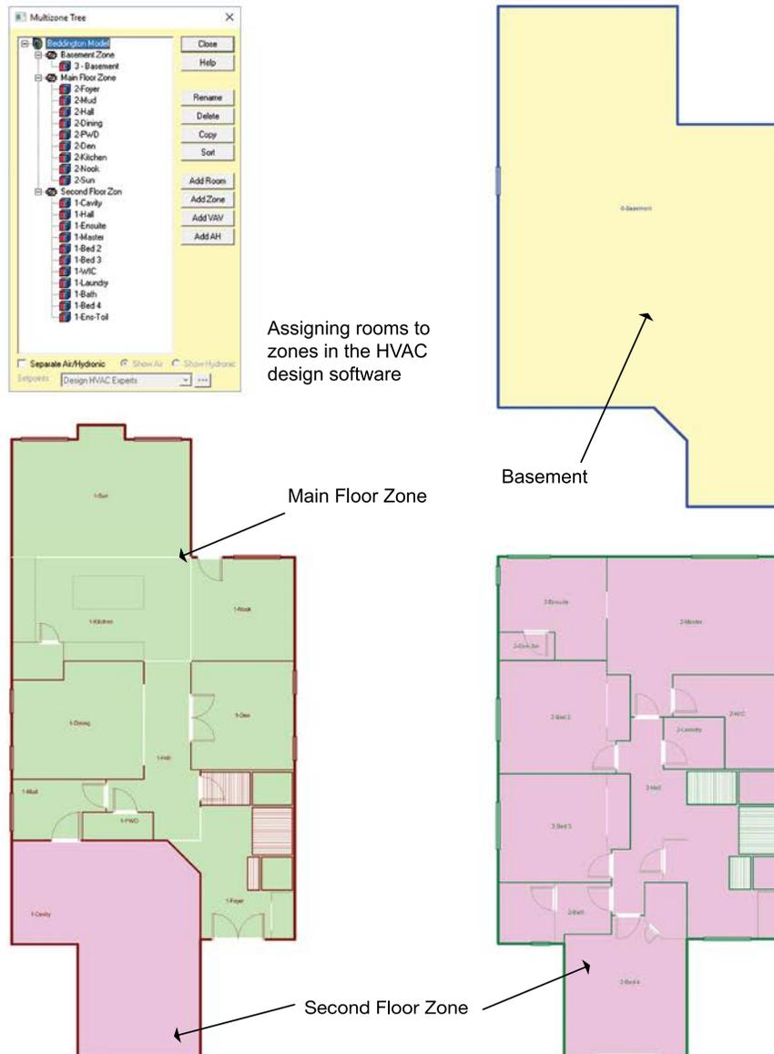
**Figure B-21:** Example of Floor-by-Floor Zoning using a Software Design Tool
