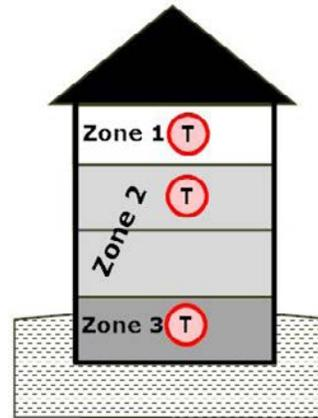
**Figure 6-3:** Thermostat Placement when a Zone has more than One Floor
