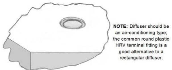
**Figure 5-3:** Ceiling Supply Outlet, shown with a Round Diffuser
