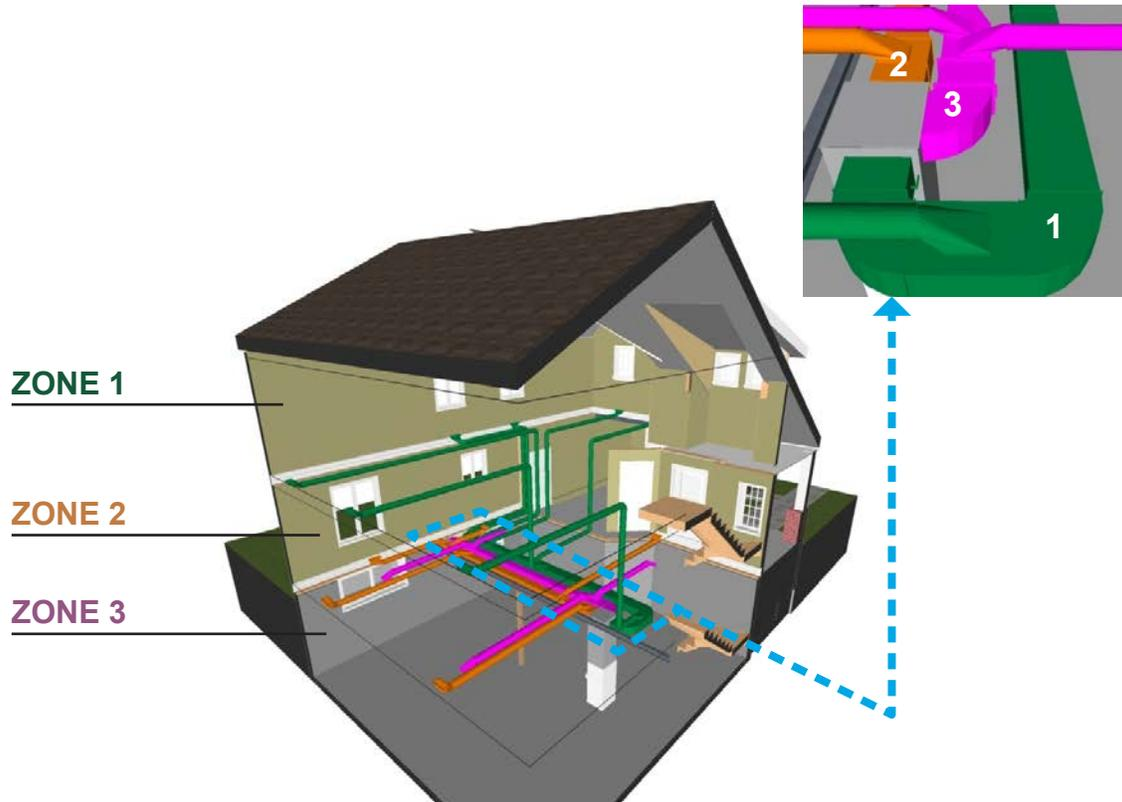
**Figure 3-1:** Floor-by-floor Zoned Ducting using OPTION A: Traditional Supply Ducts
