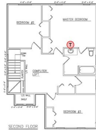
**Figure 6-2:** Thermostat Placement in the Upper-Floor Master Bedroom
