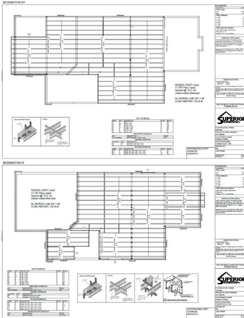
Figure A-7: Joist Plan Details to Assist with HVAC Duct Routing
