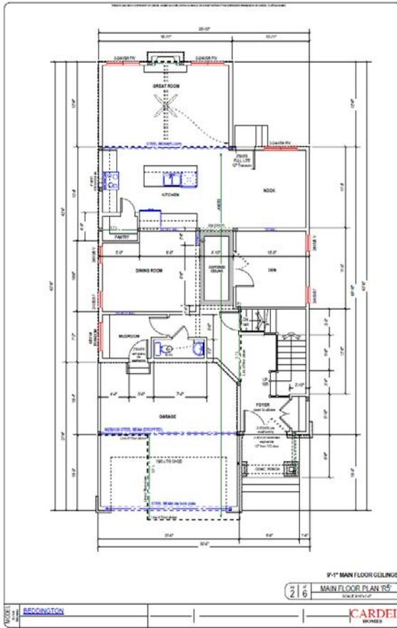
Figure B-18: Main Floor Plan
