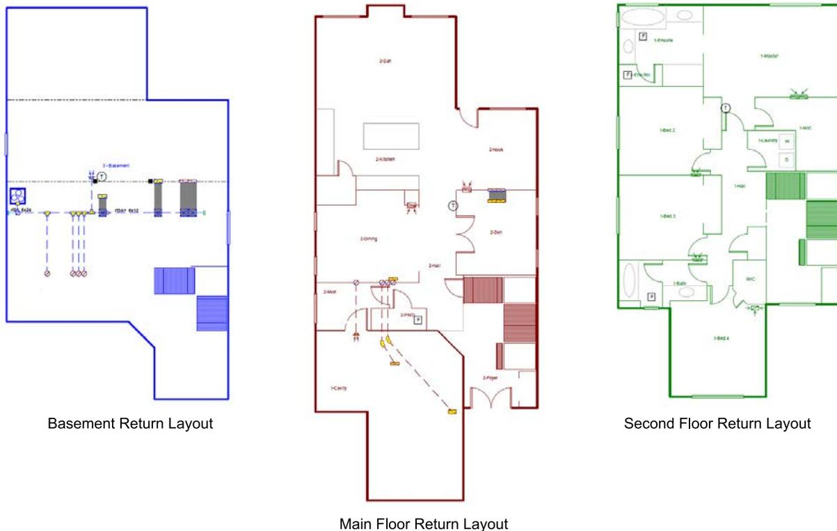
**Figure A-10:** Return duct layout for the Example Duct Design
