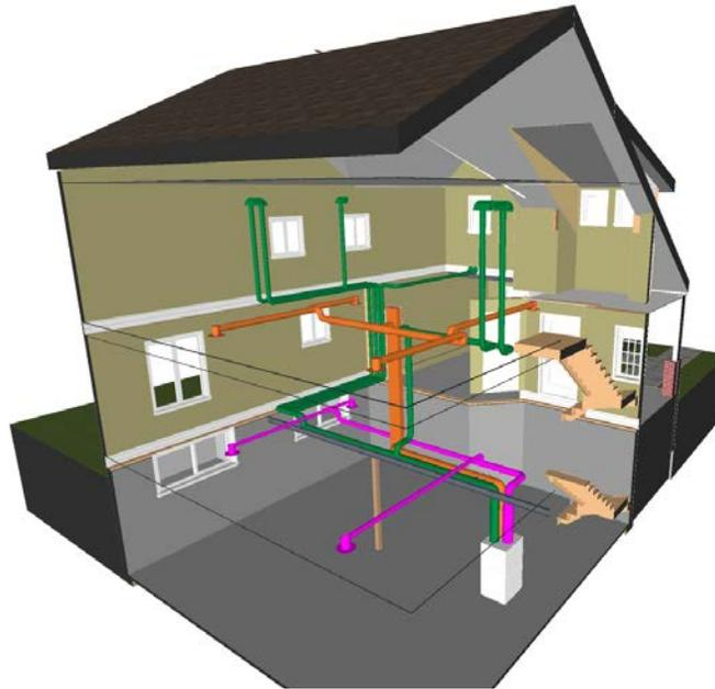
**Figure 3-2:** Floor-by-floor Zoned Ducting using OPTION B: Central Supply Ducts
