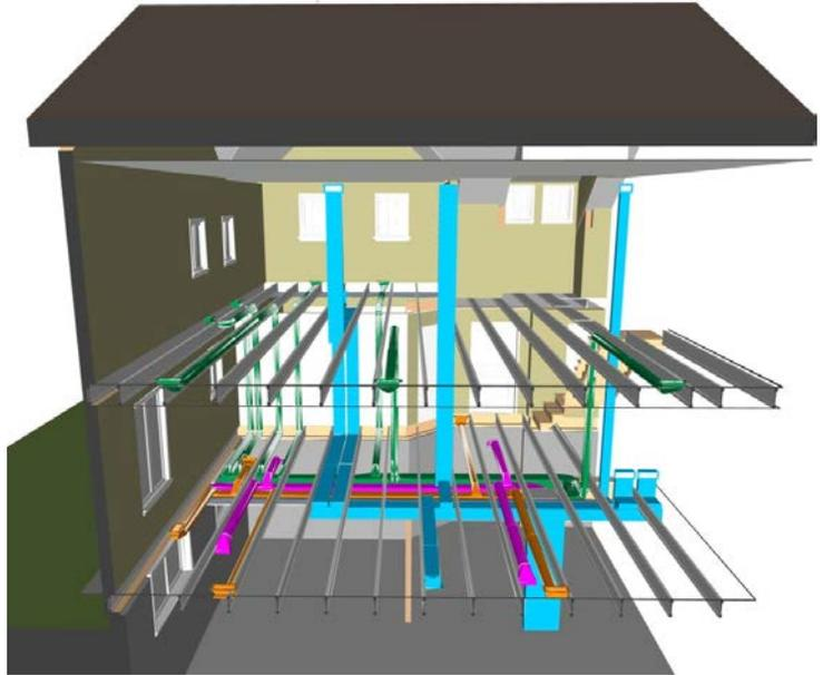
**Figure 5-6:** Example of coordinating the layout of ducts with the framing plan to minimize use of elbows
