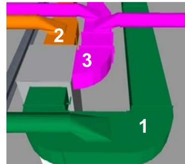
**Figure 5-5:** Each Zone has a separate supply trunk (ST)
