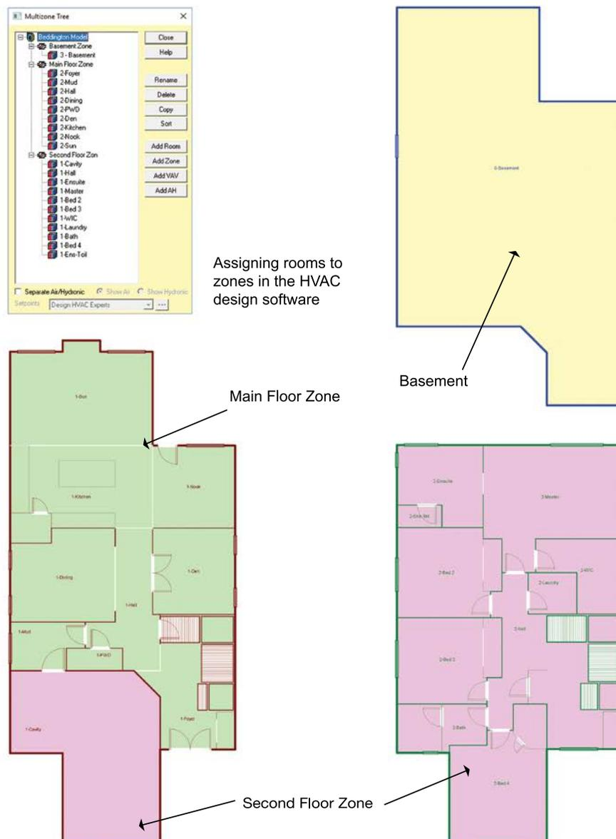
**Figure A-8:** Example of Floor-by-Floor Zoning using a Software Design Tool
