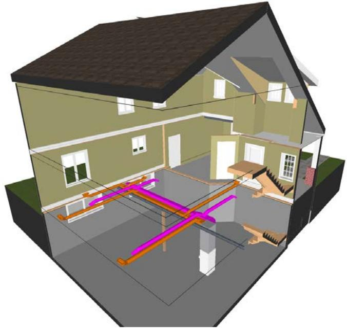
**Figure 5-10:** Supply Ducts for Basement & Main Floor Zones
