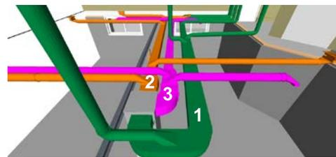
**Figure 5-11 INSERT:** Each Zone has a separate supply trunk connected to the equipment plenum (e.g. "1", "2", & "3" for second-floor, main-floor & basement zones).
