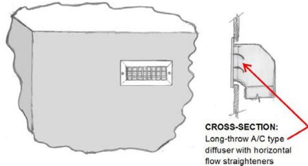
**Figure 5-2:** Interior High Wall Supply Outlet, shown with a Rectangular Diffuser
