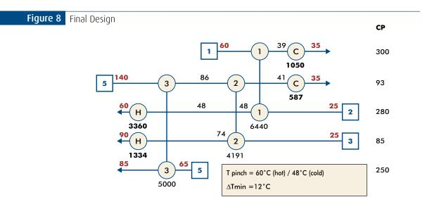
*Figure 9* presents the flowsheet obtained from the design in *Figure 8*. The new design includes three heat exchangers. The reject from the chip wash water cleaners is used to heat the paper machine showers. At the same time, the reboiler's contaminated condensate first heats the pulp washers' showers, and then, the steam plant make-up water.
