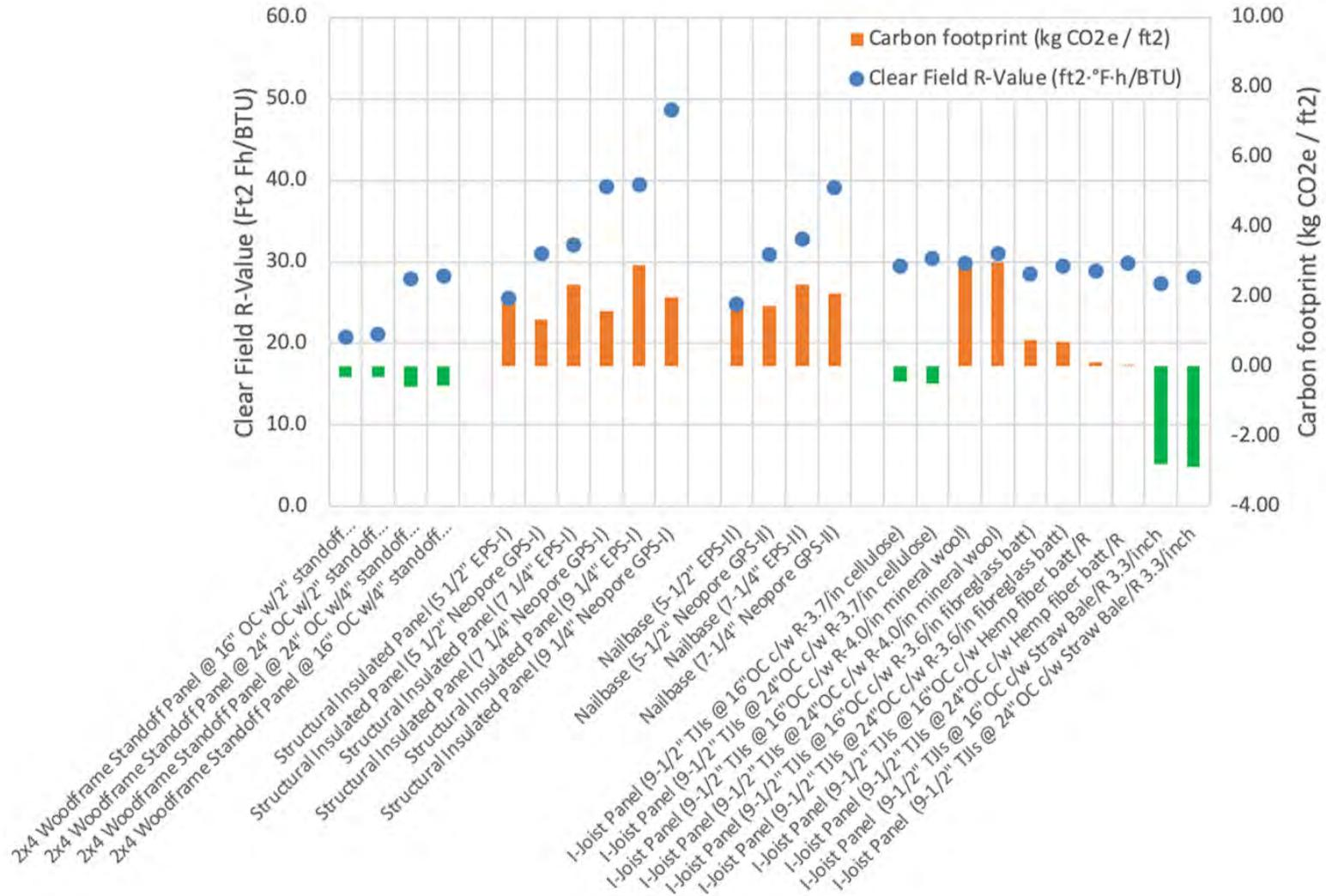
**Figure B-1:** Estimated clear Field R-value and embodied carbon content of variations of the PEER panels described in Appendix A. The blue dots represent the R-value, orange bars represent embodied carbon content per ft², green bars represent panels that are net-carbon storing. Note—cladding omitted from R-value and embodied carbon estimates.
