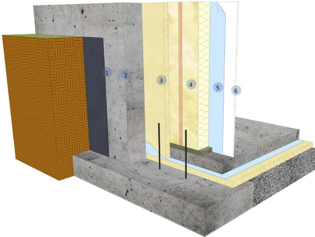
**Figure 19: Approach 2 – Example of an interior insulated foundation wall employing rigid insulation materials. Contact the local manufacturer representative for specific application details.**
