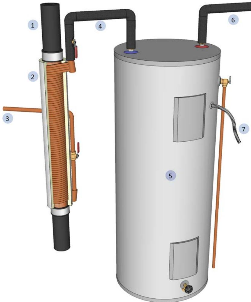
**Figure 22: Illustration of a Drain Water Heat Recovery System (DWHR)**
