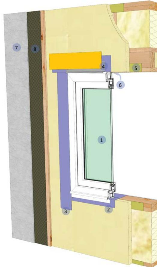
**Figure13: Builders installed flange windows and fastened through insulation into framing.**
