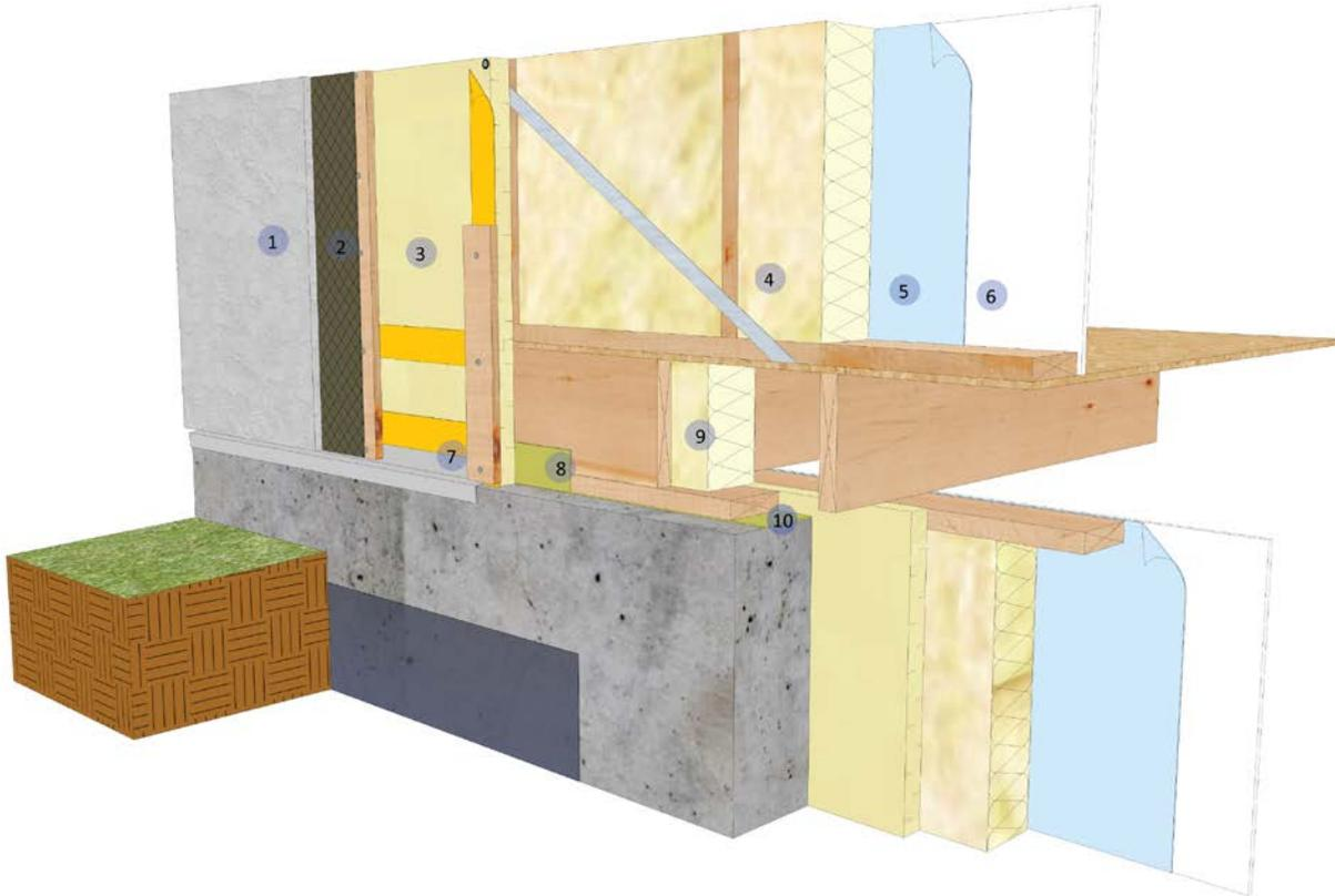
**Figure 12: Illustration of a below grade wall to above grade wall transition employing exterior insulation.**
