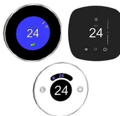
Figure 6-2: Smart thermostats automatically adapt temperature settings to improve comfort and reduce energy consumption
