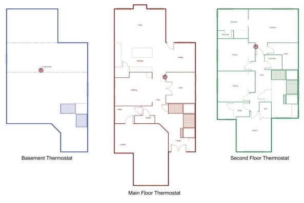
Figure A-12: Zone Thermostat Locations in the Example Three-Zone HVAC Design
