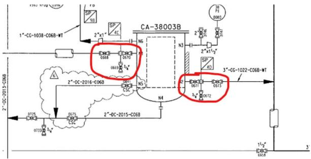
In case where there is no DBB, that Operates at >2500kpa, then regular maintenance activities would fall under the annual Turnaround-Group. And if corrective maintenance activities were required, then the system would be shut down and repaired as required.
