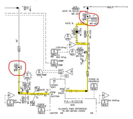
The above is only one example of many on how the TN FPSO is designed with SVI's, and how regular and corrective maintenance is carried out without plant shutdowns but still working safely. Below is a case of greater than >2500kpa whereby a DBB is required. This is a glycol utility system (glycol filters) that operates at ~5500kpa. A DDB is required to complete regular and corrective maintenance on the filter "B" without shutting the system down.
