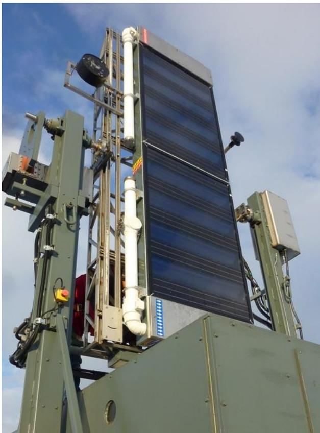
Figure 1: BIPVT collector prototype designed by KNU on CanmetENERGY’s PVT Testing Facility
