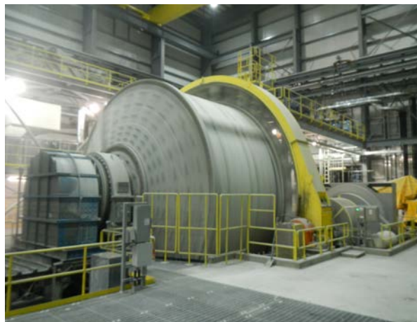
Photo: New Gold Inc. The 7,500-HP SAG mill operates in the grinding circuit.
