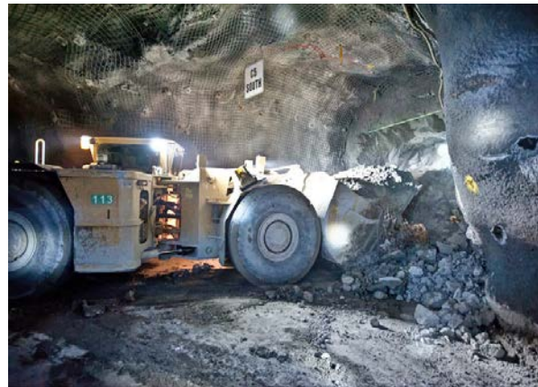
Photo: New Gold Inc. A scoop mucks out an underground draw bell. Overhead rock collapses into the draw bells to be extracted.
