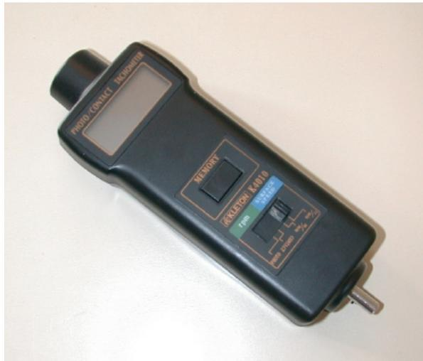
A practical tachometer for energy auditing is shown in Figure 4.13. This unit is capable of contact or non-contact measurements.
