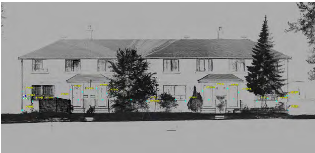
Figure 7-4: A survey control network is projected onto a point cloud to see its relative position in 3D.
