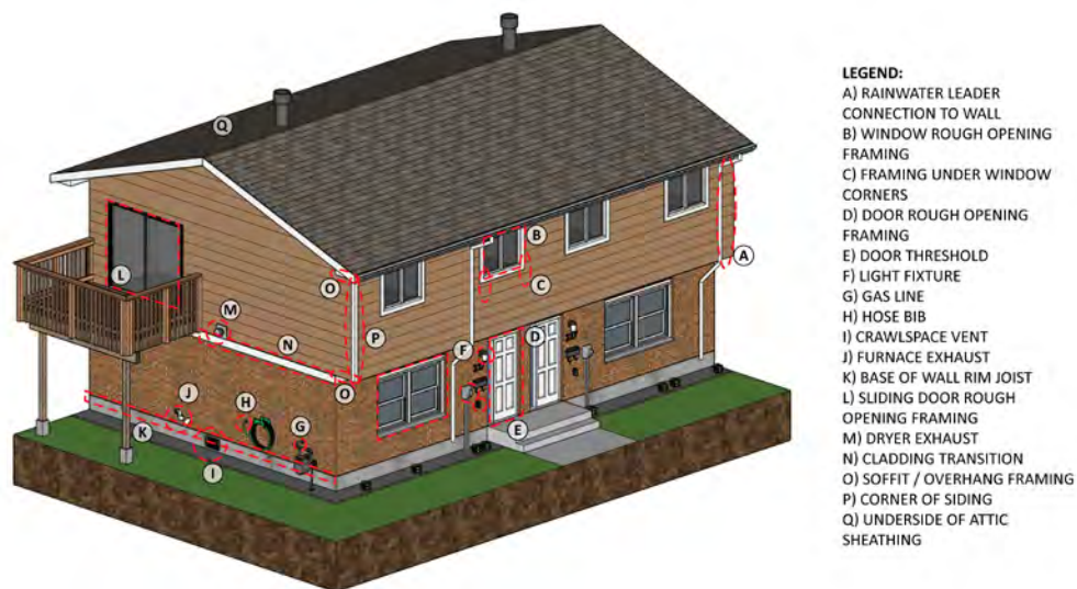
Figure 3-8: Typical locations of moisture/insect damage in building structure.
