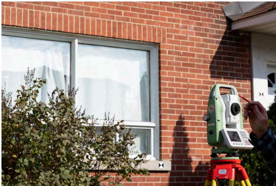
Figure 7-3: A Total Station can be used to obtain 3D coordinates of discreet points (i.e., building corners, window openings, etc.) or targets.
