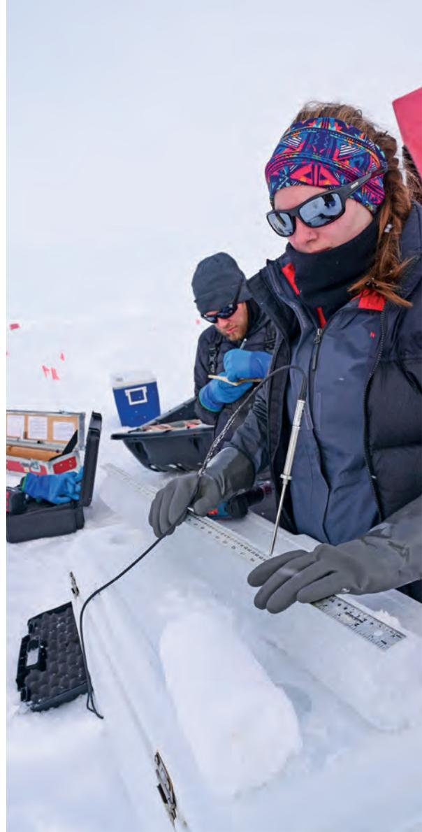
Measuring the temperature of a core of first-year sea ice
