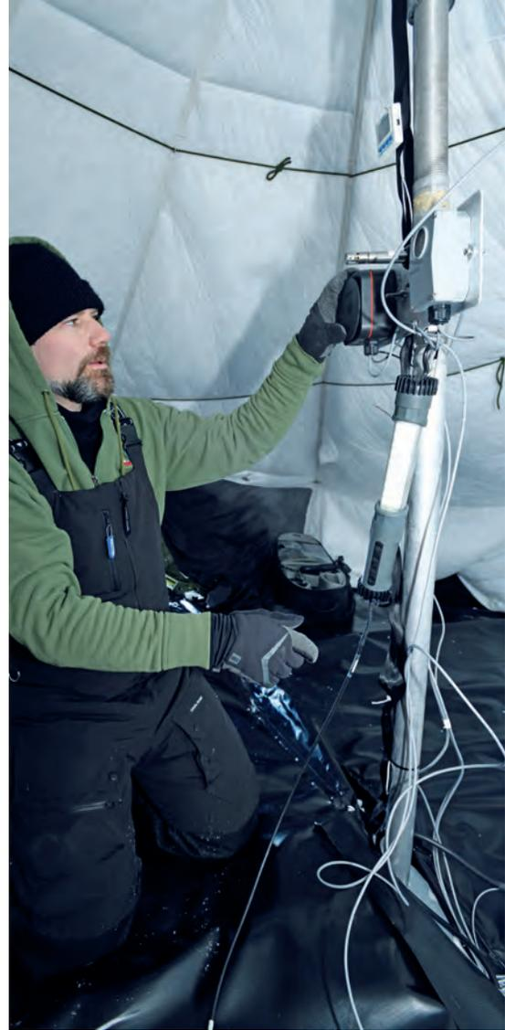
Installing temperature, carbon monoxide and carbon dioxide sensors in an experimental 10-person tent near Resolute, Nunavut
